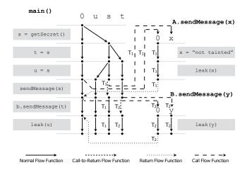
Figure 4: IFDS propagation for the example in Figure 1. Edges are labeled by the analysis task that creates them. The unlabeled edges are created by task  $T_0$ .
